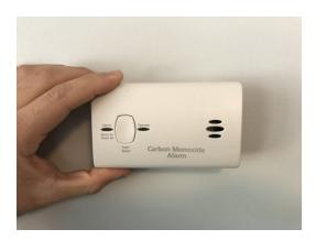
Look around your house for carbon monoxide detectors (see photo above) and push the test button on them to see if they still work. How many working carbon monoxide detectors do you have in your home?
